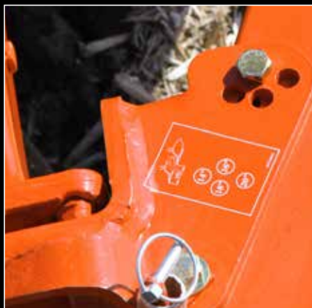
Easy manual working width adjustment for RM2000-RM2005. Only 1 bolt to reposition.
