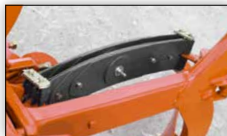
Double spring package: with 14 leaves (1400 kp)
