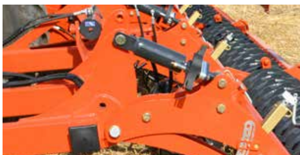
The rear depth control is adjusted via the roller equipment.
