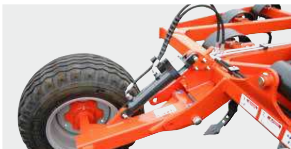
CU1000T: The front working depth is adjusted by gauge wheels.
