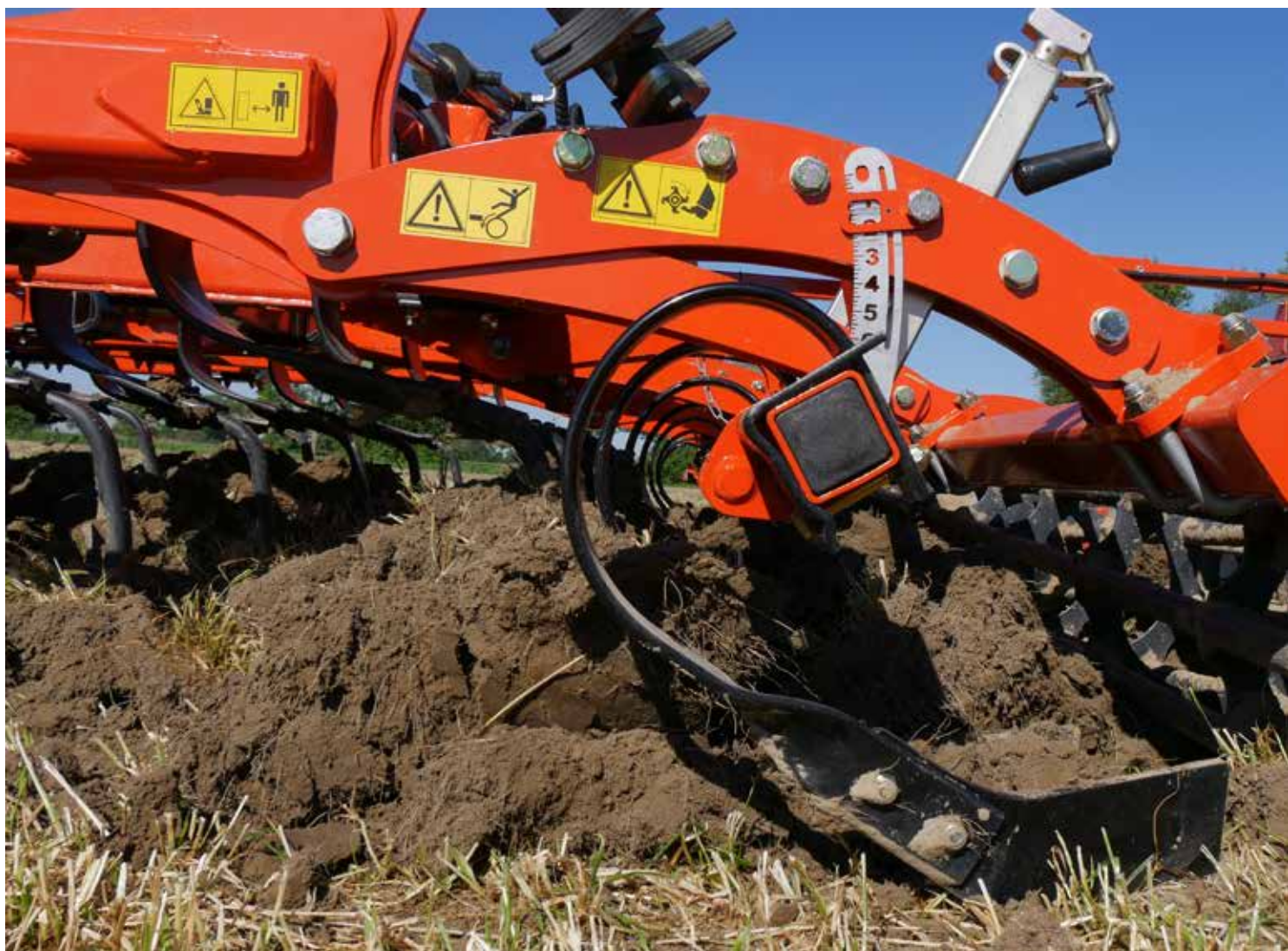
Levelling tines on light to medium soil conditions.
