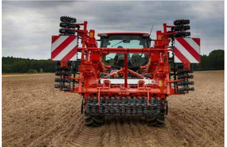
TH4400F - Safe road transport and easy hydr. folding from transport into working position. All THs are designed into three sections to follow better ground contour.
