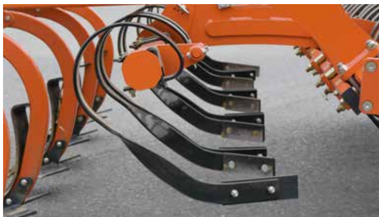
Levelling tines for light to medium soil conditions.
