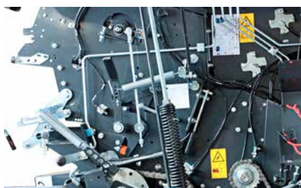
Rigid steel pipes for hydraulic circuits.
