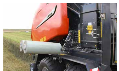
Stretch film cassette with hydraulic operation for maximum operator convenience.
