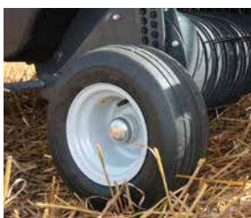
Generous flotation tyres with easy height adjustment.
