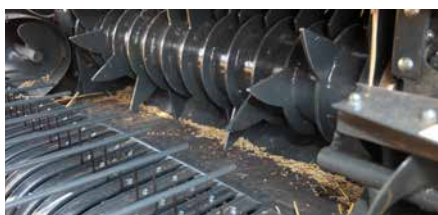
PowerFeed intake system.
