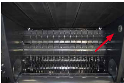
Moisture sensor located inside the bale chamber.
