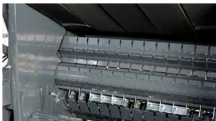
Profiled rollers provide instant bale formation and are equipped with self-cleaning scrapers designed for working in wet silage conditions.
