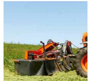
A BreakAway solution, integrated in the headstock, helps clear obstacles.
