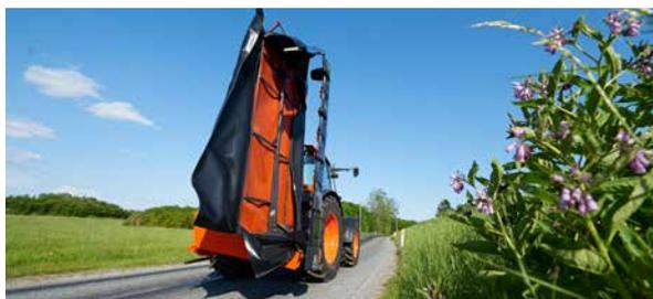
For transport the machine is folded hydraulically from the tractor cab to the vertical transport position well behind the tractor, ensuring a stable and steady transport.
