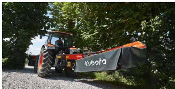
For transport the mower is swung hydraulically into horizontal position behind the tractor. Fast and easy conversion, with no need to leave the tractor.
