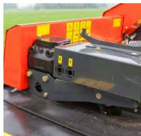
The auger is driven by a small gearbox with an additional power requirement of only 5hp.
