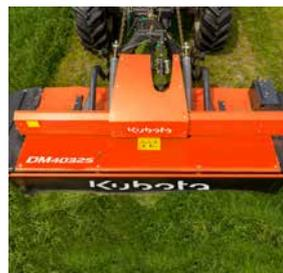
Two speed driveline is standard. Standard speed is 1000 rpm. By switching driveline pulleys 750 rpm, for reduced fuel consumption, is possible.
