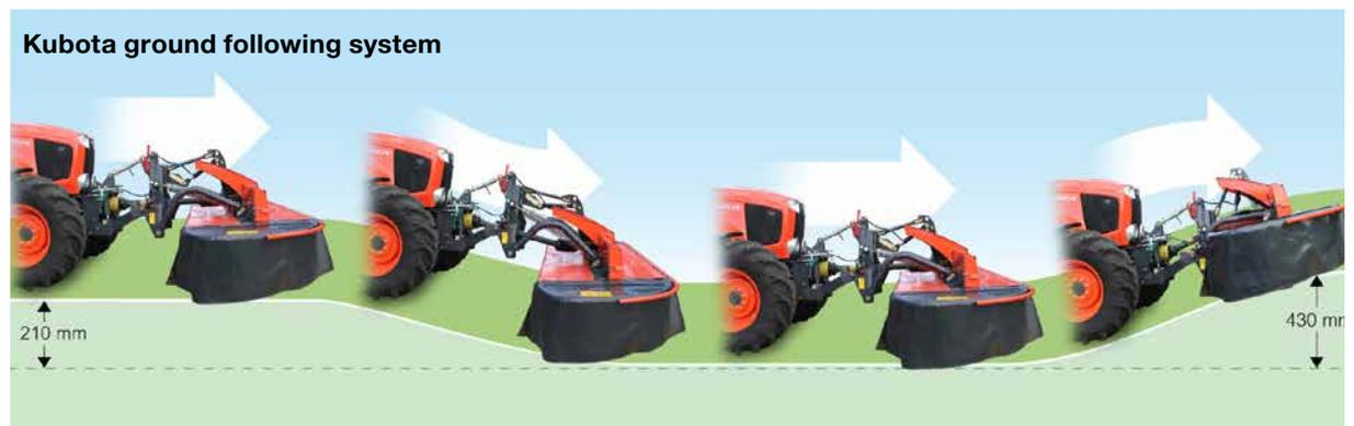
An adaptation range of 430mm upwards and 210mm downwards ensures untroubled ground following.
