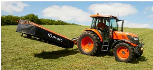
Lift on headlands via a hydraulic cylinder – no use of the 3-pt hitch is needed.
