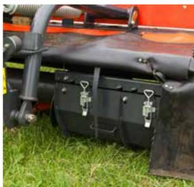
Swath width is easily changed by simply unlocking the swath plates and sliding them to the requested position.
