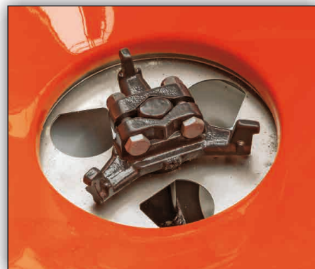
Agitator ensures even feed of the fertiliser
