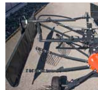
Automatic fold-able swath board with parking stand.
