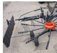
Automatic fold-able swath board with parking stand.
