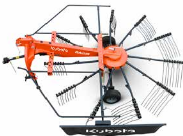
RA1039 – 3.90m working width, weighing 460kg.
