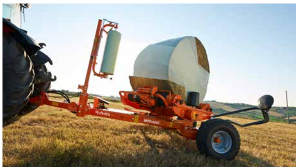
Low design of the machine ensures fast and gentle unloading of the bale.
