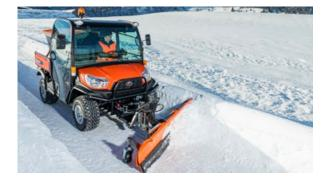
Front lifter and front cable winch
