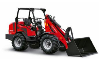
With an overall height from 2.04 m, the 3650 SLT is particularly compact.
